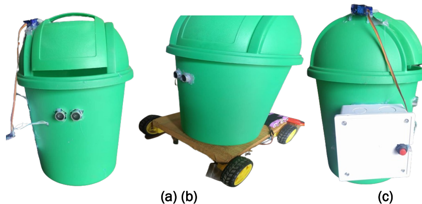
Figure 4.(a,b,c): Smartbin with ultrasonic sensor, Smartbin with bluetooth enabled autonomous system and smartbin with component case.
