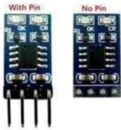
Figure 7: 5v 1A charge controller
