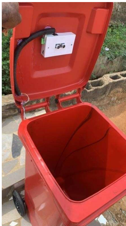
Figure 14: Smart Bin displaying the Micro-Controller
