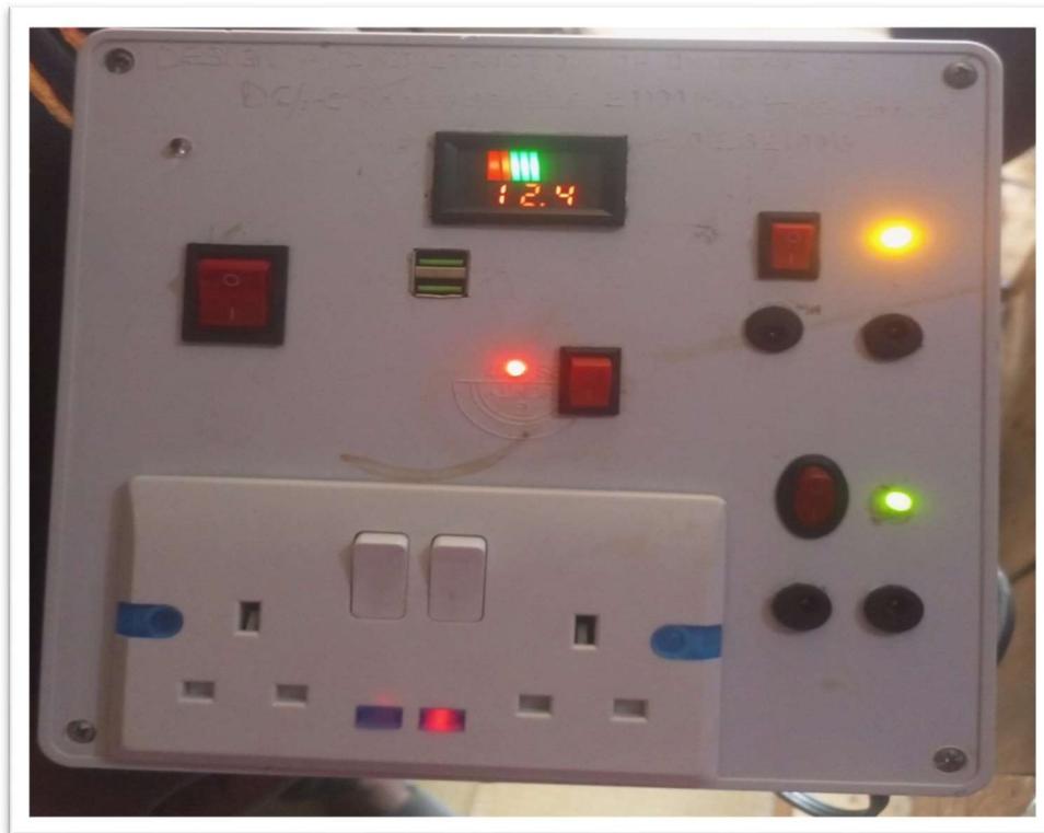
Figure 4.2e: showing the complete construction of uninterrupted DC/AC Rechargeable 30000mah power source when Powered On.
