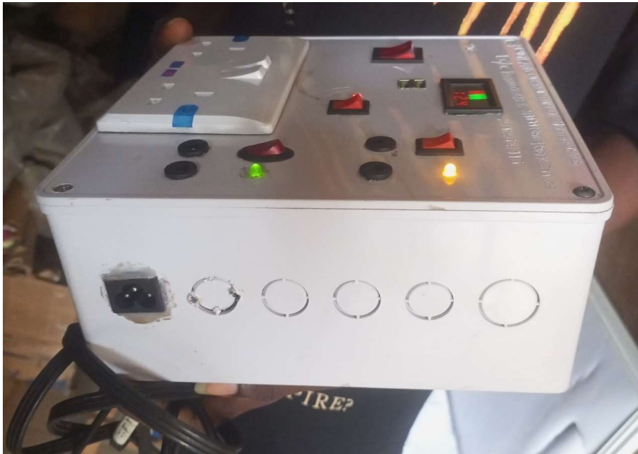
Figure 4.2d: Showing the Complete casing with IEC C6 mounted on the side for AC source charging
