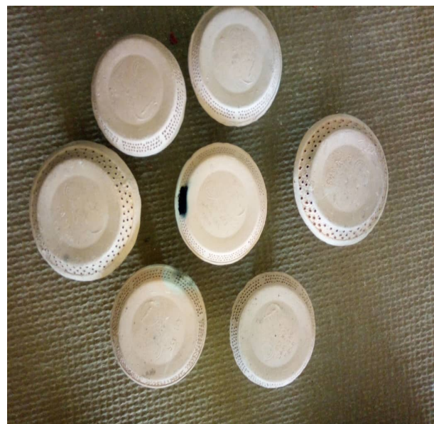
Fig 5: Stacking of burner pieces for firing
