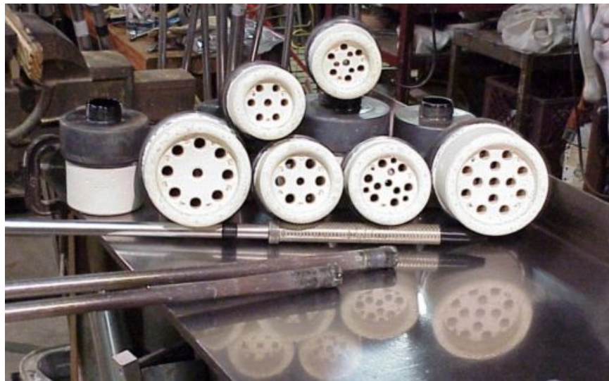
Fig 1. Ceramic burner nozzles from Wilton technologies
