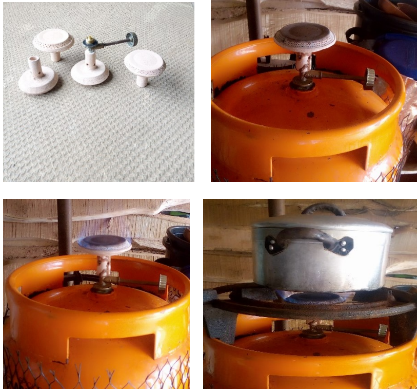
Fig. 7: In-use testing of the ceramic burner.
