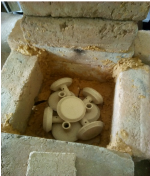
Fig 5: Stacking of burner pieces for firing
