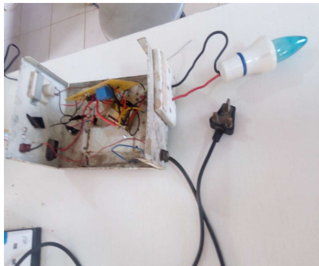
Figure 5: The Prototype setup with the testing lamp
